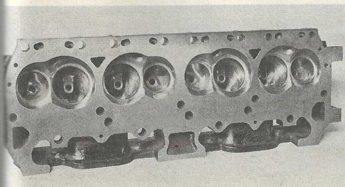
Although the engineers must have had something in mind, this constructive chamber shape could be part of the reason for the disappointing flow. Since the exhaust area is almost closed off from the spark plug, flame travel would be unusual."
