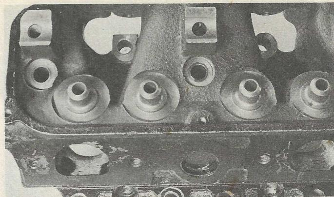
This casting has additional material on the roof of the port to allow further porting. It is possible, however, that no improvement in flow will be gained until the intake valve size is increased to 2.19 inches or larger.
