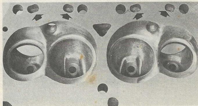
A closer view reveals the details of the W-2 chamber. Note the additional water passages to cool the area around the 10-mm taper-seat spark plugs. The piston dome required to fit this chamber and still gain a desirable compression ratio would be a dandy!
