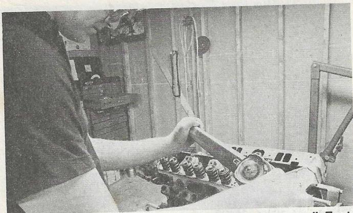
The head bolts must be tightened in several "steps." Tests have shown that if bolts are torqued in 10- or 15-ft/lb increments they will seat 1/8-1/4 turn deeper in the thread bores. This means that the head gaskets will be compressed more tightly, providing a better seal.
