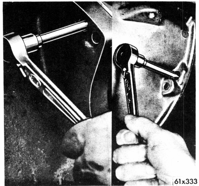
Fig. 4 – Adjusting offset dowels
