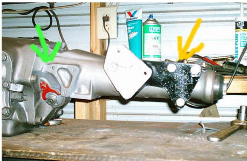
There are a few other mods required to use this adapter. The B-body mounting lugs must be ground down to keep the lugs from hitting the trans support rail (Or you can notch the support rail.) (Green arrow.) Also, you will have to give the trans tunnel a couple of dimples with a ball peen so that the adapter attaching bolts don't jam against the tunnel. (Yellow Arrow.)
