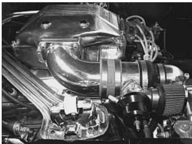
Fig 9-c / Passenger side discharge duct.
