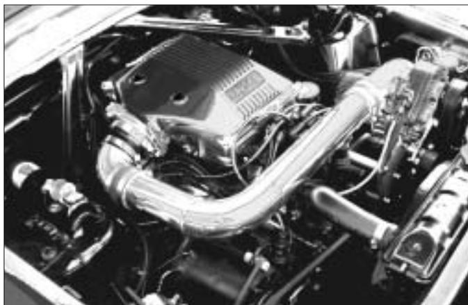
Fig 9-b / Driver side discharge duct.
