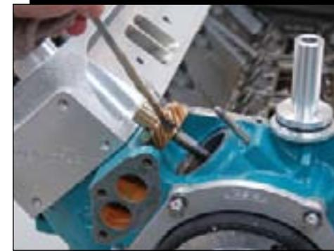
A dab of grease on the bronze gear is a good idea during assembly. A bronze gear is required when using a steel (not chilled iron) camshaft. Milodon supplied the standard length bronze gear for this engine.
