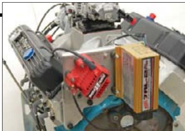
We prefer to use our own ignition system on the dyno so a plate was made to hold it on the back of the engine. High end parts from MSD supply a lot of juice to the plug. This is the same setup that we use on high compression race motors so it might be overkill for this engine.
