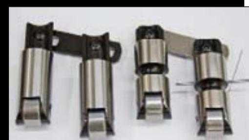
**RIGHT:** One old time hot rodder trick is to use AMC lifters in a Chrysler engine. The AMC lifter on the right has pushrod oiling as well as pin oiling while the standard Chrysler lifter on the left has neither. The AMC lifter is Comp part number 848, the Mopar lifter is a Comp 829.
