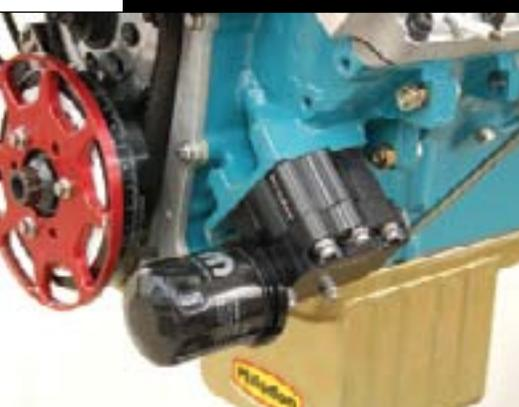
The tiny "teacup" oil filter is handy when priming the engine since it doesn't hold a lot of oil. We're running a System One screen type of filter (which E-Booger isn't fond of) on the dyno so this little filter is just for assembly and transport. The Milodon billet oil pump assembly saves a few pounds and looks great.
