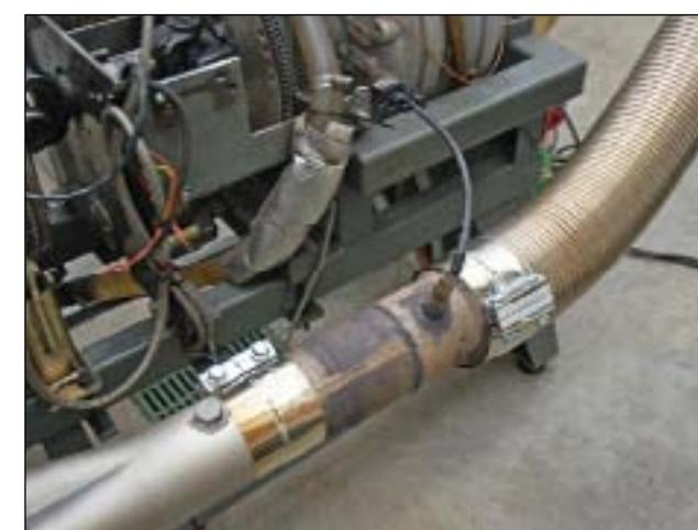
Wide band O2 sensors in each exhaust pipe keep track of the air fuel ratio during the dyno tests. Running unleaded fuel is a bonus for the dyno operator since there isn't any lead to foul the O2 sensors.
