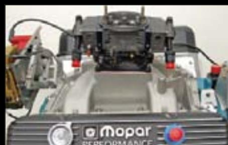
**RIGHT:** Baseline testing was done with a new Holley 850 Ultra XP. Part number for the Ultra XP version is 80804. These newest carbs from Holley are fully adjustable including idle airflow as well as jetting on all circuits. The new Ultra XP carbs also include larger fuel bowls with O-ring inlets, bowl drains, adjustable linkage and lightweight all aluminum construction. All testing was run with the Mopar M1 4500 intake manifold and a Wilson adapter.
