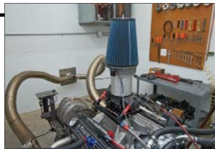
The dyno cell at Gray's Automotive is equipped with a mass air flow sensor as well as fuel turbines so both airflow and fuel consumption can be measured. Keeping track of these two items allows many of the other measurements such as BSFC and volumetric efficiency to be calculated.
