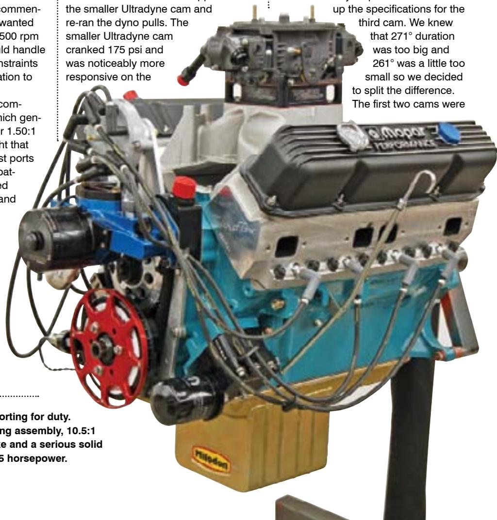
Low deck 470 CID engine reporting for duty. Trick Flow heads, SCAT rotating assembly, 10.5:1 compression, Mopar M1 intake and a serious solid roller camshaft adds up to 685 horsepower.
