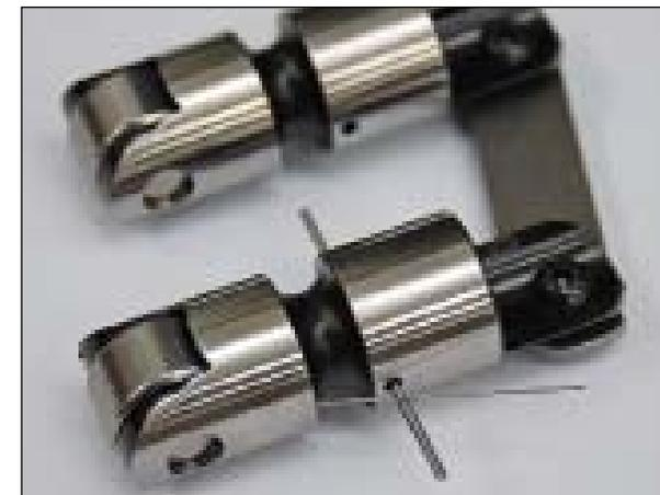
**ABOVE:** A close up view of the Comp 848 AMC lifter shows the oil passages. High pressure oil is fed from the gallery down to the pin via the small angled hole. The larger hole picks up low pressure oil from the lifter side clearance and directs it up to the pushrod cup. These AMC lifters work just fine in a stock block as long as the lobe lift isn't too large. We didn't have any oil pressure problems at 0.460" lobe lift but we were probably close to the limit.
