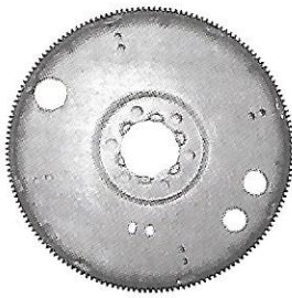
FW301 164 Teeth, w/o Weight (Domed) 13 13/16" Diameter 3232138
