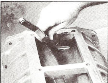
Clearance between the rotors and the end plate should be .018 to .020-inch maximum at the rear, .008 to .010-inch at the front. However, these measurements are not critical if the blower is to be rebuilt.
