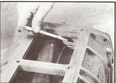
Visually inspect both end plates for wear or deep scratches.
