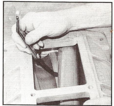
Finally, check the rotor-to-rotor (C and CC) clearance up the middle. This is a difficult measurement to make if you aren't used to the "feel" of the fit of the gauge between the rotors. You want to measure the clearance at the leading and the trailing edge of each rotor lobe, which should be approximately .020-inch each, or a total of .040-inch. If the total of both the C and CC clearances for any lobe is more than .060-inch, the blower is worn out and not worth buying.
