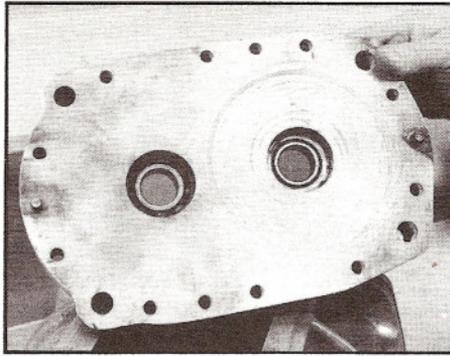
If an end plate is gouged like this one, the blower is not fit for use as-is. However, both the end plate and the end of the rotor (which would also be worn) could be machined smooth again when the blower is rebuilt, so this is not a serious problem...provided the rest of the rotors, and the case, are not worn.
