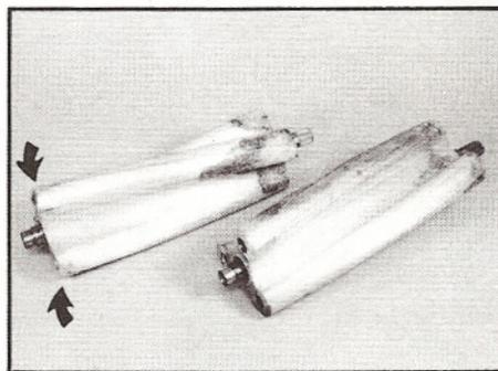
Once you clean the grime off of diesel rotors, you might find surprises like this. This 6-71 blower apparently sat outside for some time, and collected water in it, which corroded the aluminum rotors at one end. And at the other end, some very bad bearings allowed the tips of the lobes to be severely worn away (arrows). These rotors are complete junk.
