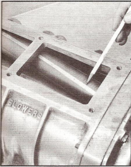
Most people first look at the outer edge of the rotor lobe, but this is usually not where wear is first noticeable (the rotors will usually hit each other before they rub on the case wall). The outer lip, or flat raised edge, of the rotor should be at least .080 to .090-inch tall and should not have any major gouges or dings in it. This one is passable.
