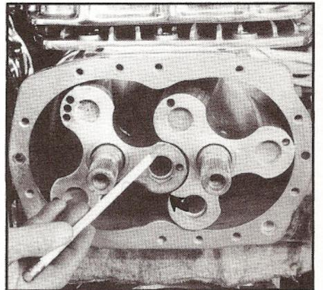
On this open blower, Don shows where the clearance between rotors is measured, with the rotors positioned as shown. Then the left rotor would have to be rotated all the way around to measure the other side of the same lobe (arrow), and the feeler gauge would have to be inserted from the right side. If it sounds confusing (and it can be), see if you can take the blower to a shop to have it checked before you put your cash on the table.
