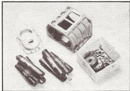
If you're going to have the blower rebuilt (which is the smartest approach), you might as well buy a good, stock, used core off of a diesel, like this 4-71, rather than paying for a supposedly “prepped” performance blower. However, note the oil on these rotors and the inside of the case.
