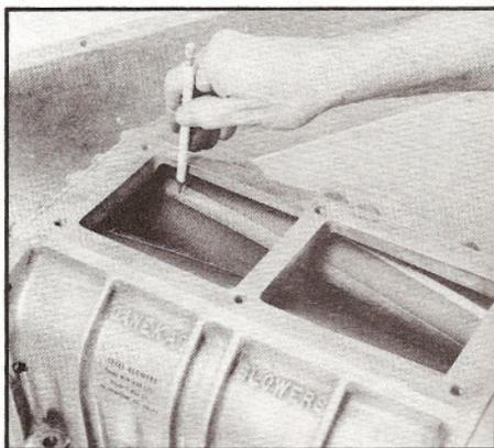
Hampton suggests you be very wary of used race blowers, since they are constantly subjected to severe operating conditions, and most aren't put up for sale until they are no longer rebuildable. One of the first places to check for damage on any blower is the sealing edge of the rotors, as shown. These are gouged and worn.
