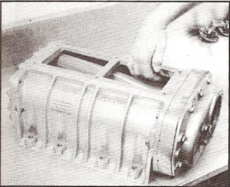
Backfires are the nemesis of any blower, but especially one from a fueler. A backfire will force the rotors up in the case, causing them to hit the case wall along the top. Feel with your hand along the inner wall near the inlet opening, as shown, to feel for gouges or wear caused by backfire. This blower failed this test. In fact, its rotors have been severely warped by a backfire sometime in the past.
