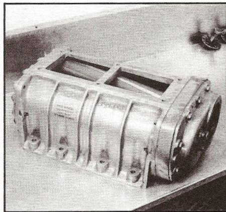
As an example of a typical used blower, Don Hampton picked this old Danekas race 6-71. Begin with a complete visual inspection of the case, end plates, and rotors looking for cracks, obvious warpage, or stripped bolt holes. This one appears fine...but appearances can be deceiving.
