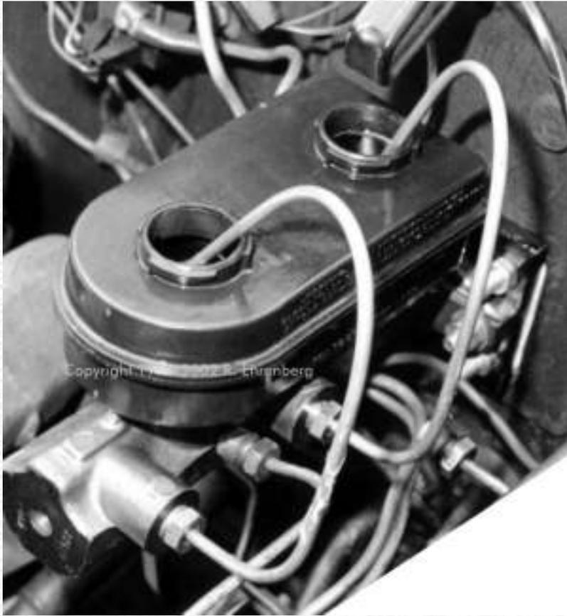
Whichever master cylinder you choose, it must be "bench" bled. This is actually way easier to do on the car. All you need are a set of homemade bleeder tubes. Pump very slowly, to the floor, at least 12 times. An even easier, though sloppier, way to accomplish the same task is to hook up the car's lines, then use each fitting as you would a bleeder screw. Requires an assistant. Makes a mess.
