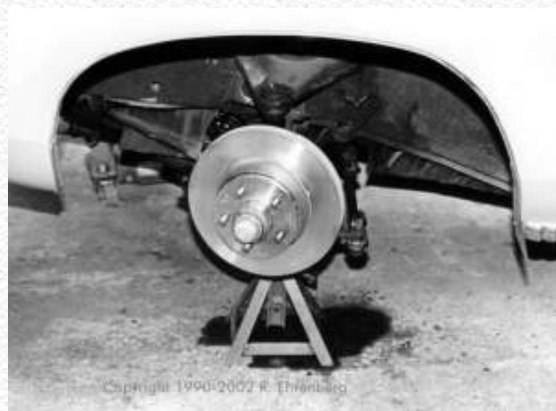
. Real, visible progress! We've installed the rotors, adjusted the bearings, and installed the dust new dust cap. With discs, there must be zero end play. Tighten until the play just disappear, then a skosh more.
