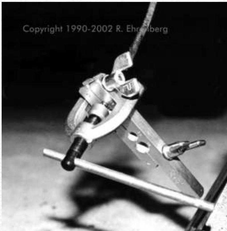
Unwind and discard about one inch of armor from each of the cut ends, and double flare the tubing, using a tool such as this. The ends must look like the drawing when you're done. And - remember to slide the tubing nuts on before you flare the ends!
