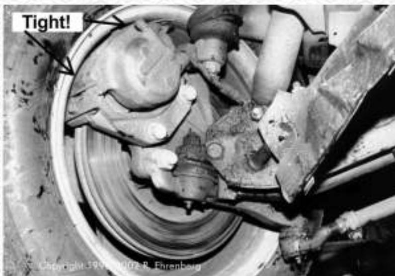
Here's the fat rotor, 15-in wheel setup from the rear. As you can see, no way are 14-in. wheels gonna clear this setup.
