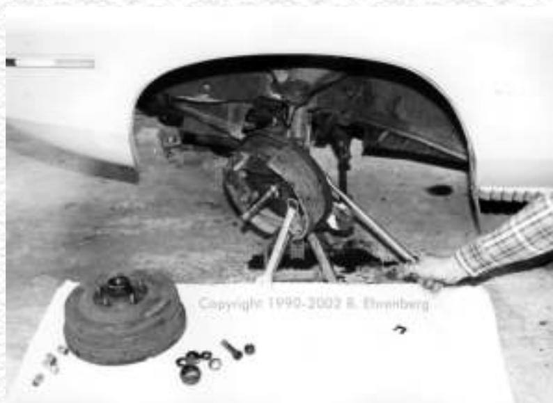
Pull the old stuff off the car, and the teardown is complete. Of course, if you plan on doing any additional front-end work, now's the time!
