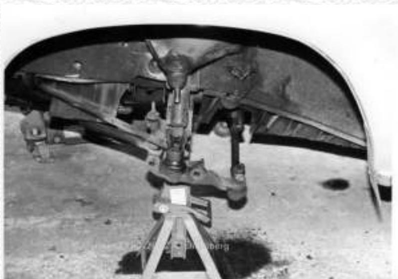
New knuckle bolts in place exactly the same way as the old one came off. Re-use the old ball joint bolts, with thread locking compound, torqued to
