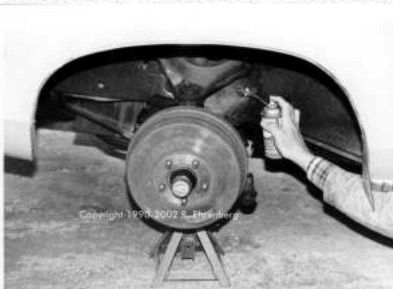
Let the games begin! Step one, after safely supporting the vehicle on stands, is to soak the hose fitting with rust penetrant. Then unscrew the hose fitting and remove the retaining clip
