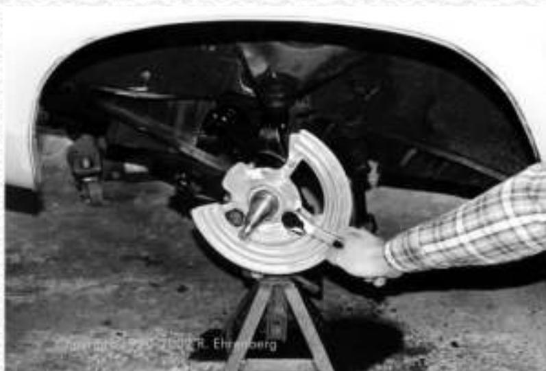
Pack the wheel bearings in the usual way, and install the seal. Mopar hi-temp lube (p/n 4318064) is the ticket!
